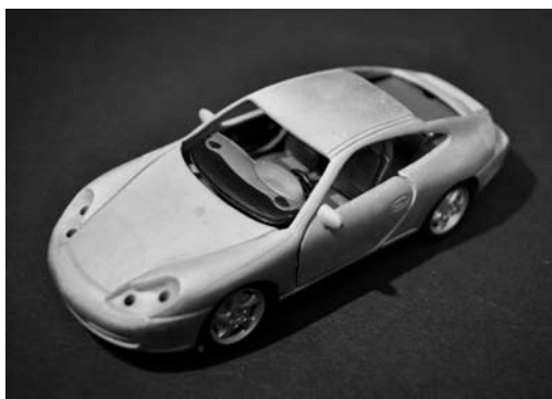
Figure 1 Aluminium deposition on a toy car
